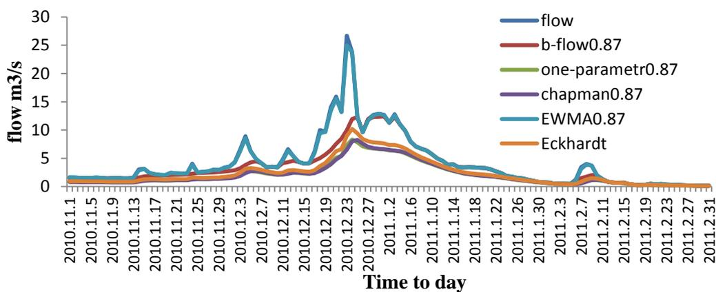
**Fig 6.** Separation of flow hydrograph with B-Flow, One-parameter, Chapman, EWMA, and Eckhardt methods at Arazkouseh Station in the part of water Year (2009-2010)
