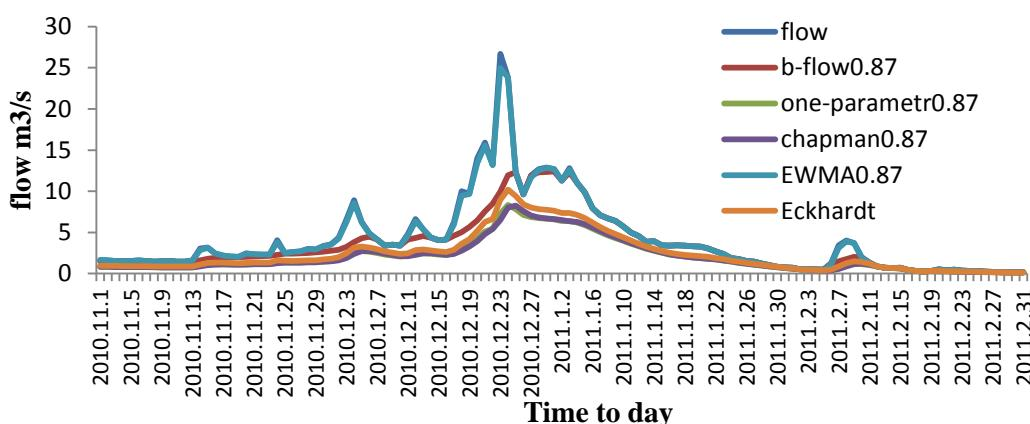
**Fig 6.** Separation of flow hydrograph with B-Flow, One-parameter, Chapman, EWMA, and Eckhardt methods at Arazkouse Station in the part of water Year (2009-2010)
