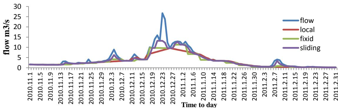
**Fig 5.** Separation of flow hydrograph with Hyslop and Eckhardt methods at Arazkouseh Station in the part of water Year (2009-2010)
