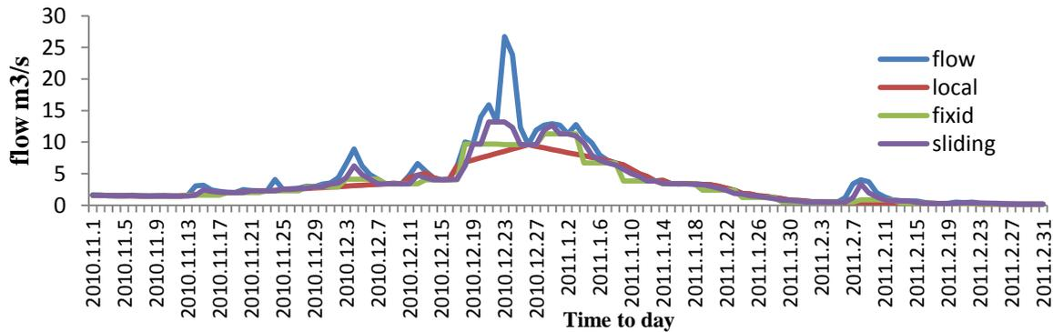
**Fig 5.** Separation of flow hydrograph with Hyslop and Eckhardt methods at Arazkouse Station in the part of water Year (2009-2010)
