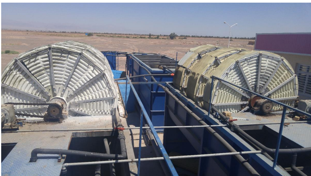
Fig. 3. The rotating disks in the RBC case study
