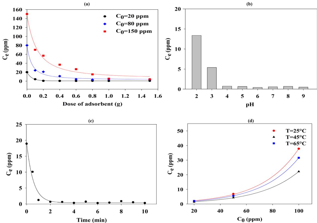
**Fig. 4.** (a) Effect of initial concentration at different sorbent dosages (T = 25 °C and 10 min), (b) Effect of pH on Cd<sup>2+</sup> removal (initial Cd<sup>2+</sup> concentration = 20 mg/L, T = 25 °C, and 10 min), (c) Effect of contact time (initial Cd<sup>2+</sup> concentration = 20 mg/L, T = 25 °C, and pH = 7.0), and (d) Effect of temperature on the Cd<sup>2+</sup> adsorption (initial Cd<sup>2+</sup> concentration = 20 mg/L, pH = 7.0)
