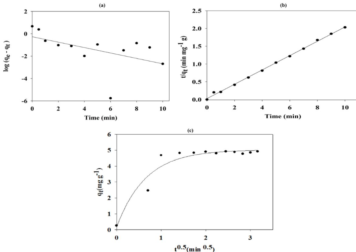
**Fig. 5.** Fitting the experimental data of  $Cd^{2+}$  adsorption onto acetone/ $H_2O_2$ -treated pistachio green hulls (sorbent dosage = 0.2 g, pH = 7.0, and  $T = 25$  °C) by (a) pseudo-first-order kinetics model, (b) pseudo-second-order kinetics model, and (c) intra-particle diffusion model
