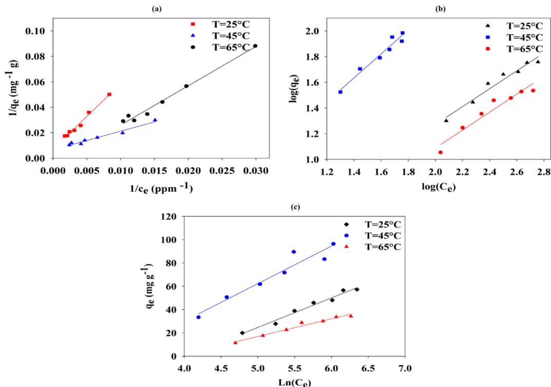
**Fig. 6.** Fitting the equilibrium experimental data of  $\text{Cd}^{2+}$  adsorption onto acetone/ $\text{H}_2\text{O}_2$ -treated pistachio green hulls at different temperatures with a) Langmuir model, b) Freundlich model, and c) Temkin model
