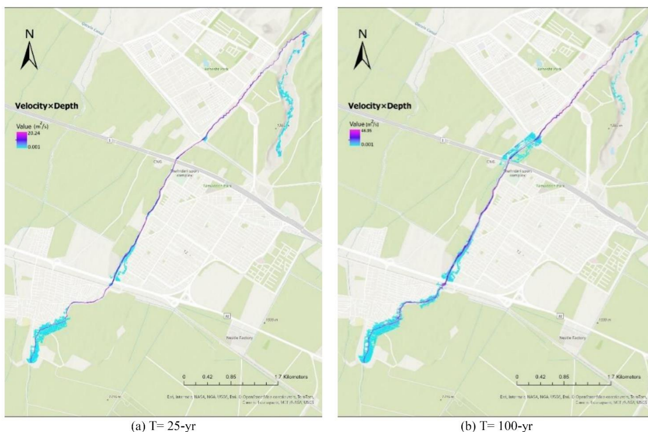
Fig. 6. Flood severity as hazard map with return period 25-yr (a) and 100-yr (b) obtained by product of flood depth and velocity data layers.
